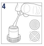
Clean the lens by using the tip of the cotton swap or lens paper\*. When cleaning a large lens surface, wipe with little pressure from the centre towards the periphery in a circular motion, do not use zig-zag motion. Discard each lens paper or cotton swap after a single use
