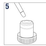
Wait until the cleaning fluid is evapourated, or speed up this process by using pressurized dry air
