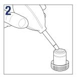
To prevent scratches on coatings and optical glass, first try to remove dirt and dust that sticks to the optical surface with an airblower or pressurized dry air (oilfree and under moderate pressure version only)
