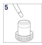
Wait until the cleaning fluid is evapourated, or speed up this process by using pressurized dry air
