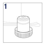
Place your objective or eyepiece on a secure location. One can use the objective's cap or eyepieces can be placed in the cut-outs within the storage box. Condensers and collector lenses can remain on the microscope
