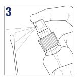
Use an absorbent lens paper or cotton swap. Damp a swap or towel with a small amount of lens cleaning fluid or cleaning mixture (Either pure isopropanol or a mixture of 7 parts ether and 3 parts alcohol)
