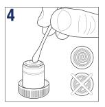
Clean the lens by using the tip of the cotton swap or lens paper\*. When cleaning a large lens surface, wipe with little pressure from the centre towards the periphery in a circular motion, do not use zig-zag motion. Discard each lens paper or cotton swap after a single use
